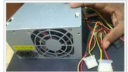
A 450 Watt SMPS for use in personal computers with the power input, fan, and output cords visible ↗
