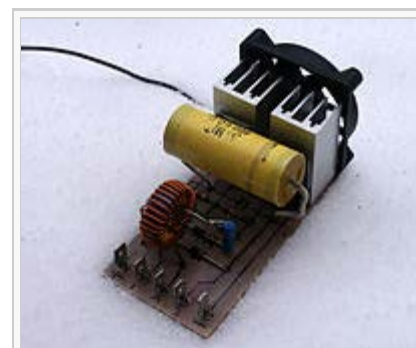
Zero voltage switched power supplies require only small heatsinks as little energy is lost as heat. This allows them to be small. This ZVS can deliver more than 1 kilowatt. Transformer is not shown.
